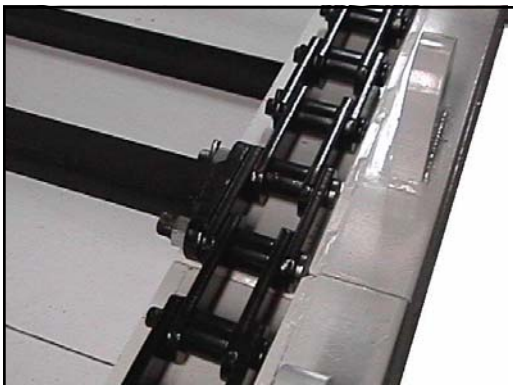
3.075" Pitch 40,000 lb. chain with solid AR-200 flights for longer life and prevents flight bending
